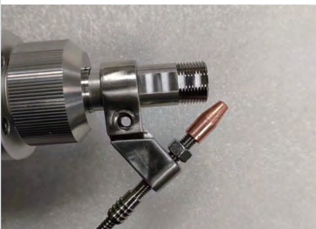
Step 3: Reinstall the copper nozzle tip and adjust the wire feed guide nozzle to a proper position
