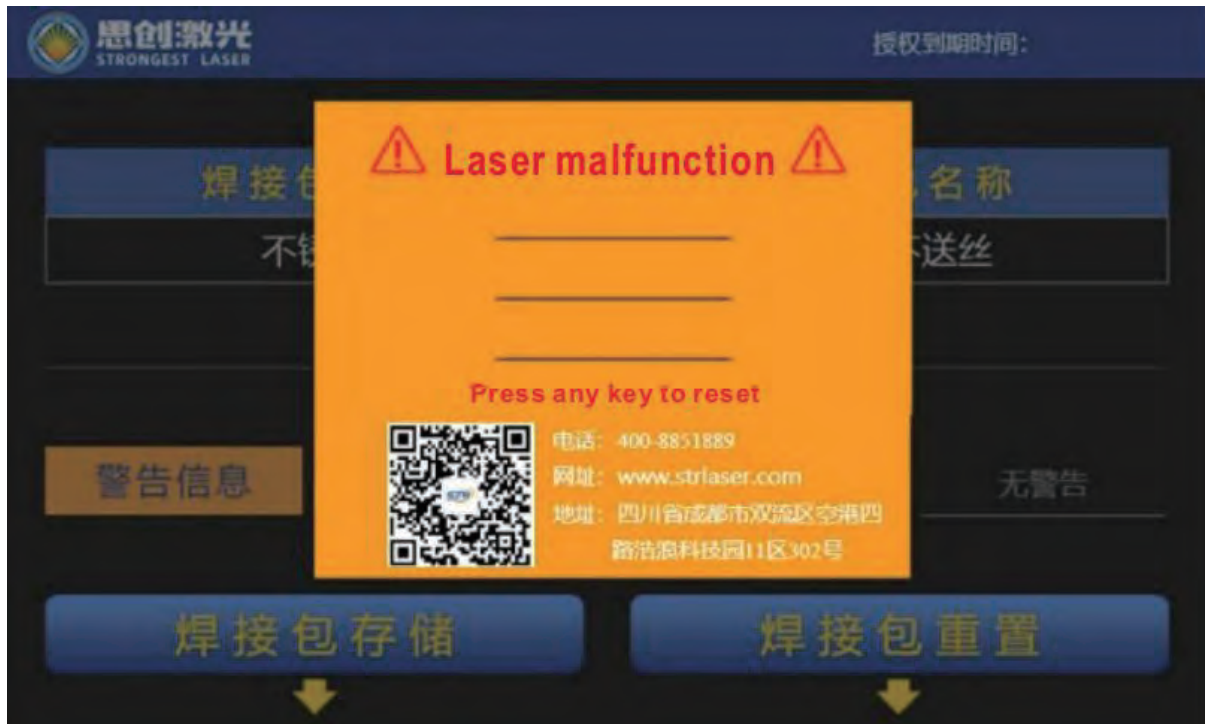
Figure 8-1 Fault Displayed on LCD
